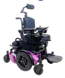
**Description**: Alltrack P3 Mid Wheel Drive (MWD) power wheelchair. Base width: 535mm. Base length: 890mm. Seat to floor height: 445mm. Turning radius: 510mm. Speed: 10km/h. Battery capacity: 50amps. Selections of: Power Tilt 50°, Power elevate 11in, Power recline with mechanical shear reduction seating functions, and Powered centre mount (PCM) elevating and articulating leg rest with flip-up, angle adjustable footplates.
