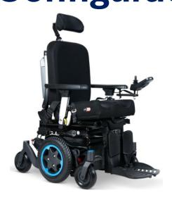
**Description**: Q500M MWD Powerchair. Includes Adjustable Seat, Armrests & Footrests. 13in Drive Wheels. 7in Castors. 60 Ah Batteries. 10km Speed. 40km Range. Options: 50 Degree Posterior Tilt. 30cm Seat Elevate. 130 Degree Recline. Swing Away Angle Adjustable Footplates or Centre-mount (CM) Footrests.
