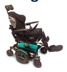
**Description**: TA iQ Mid Wheel Drive (MWD) power wheelchair - Tilt/recline/Elevate (TRE) /Leg Elevate (Centre Mount). Base width: 630mm. Base length (without footplates): 910mm. Seat to floor height: 380mm. Turning radius: 450mm. Speed: 12.5km/h. Battery capacity: 80amps. Selections of: Tilt 45°. Backrest recline with mechanical shear reduction. Seat Elevate 11.8in. Powered centre mount (PCM) elevating and articulating legrest with flip up, angle adjustable footplates (2 individual pieces).
