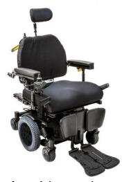
**Description**: A heavy duty powerchair engineered to meet the performance needs of the most active user. 14in Drive Wheels. 6in Solid Castor Wheels Front. 6in Solid Castor Wheels Rear. Min Seat to Floor Height 17.75in. Maximum Rate Slope 7.5°. Max Speed 7.5km/h. Selections of: Power tilt, recline, elevate (TRE) and power elevating centre mount (PCM) leg rest.
