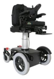
**Description**: TA iQ Junior Front Wheel Drive (FWD) power wheelchair. Base width: 600mm. Base length (without footplates): 820mm. Seat to floor height: 380mm. Turning radius: 450mm. Speed: 12.5km/h. Battery capacity: 80amps. Selections of: Power tilt 45°, Power elevate 11.8in, Power recline with mechanical shear reduction, and Powered centre mount (PCM) elevating and articulating leg rest with flip-up, angle adjustable footplates.
