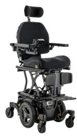
**Description**: The narrowest, most compact and manoeuvrable power base in the Quantum range. 14in Drive Wheels. 5in Solid Castor Wheels Front. 6in Solid Castor Wheels Rear. Min Seat to Floor Height 17.5in. Maximum Rate Slope 6°. Max Speed 10km/h. Mid-Wheel Drive (MWD). Q-Logic 3 Expandable Electronics. SRS Suspension. High Efficiency And Mileage. 2 Pole Motor. Fender lights. Selections of: Power tilt. Power tilt and elevate. Power Tilt and Recline.
