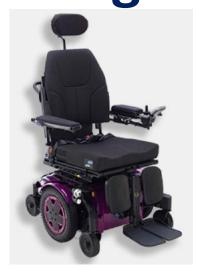
**Description**: TDXSP2 Narrow or Wide Mid wheel drive (MWD) base, Selections of: Tilt, Recline, Elevate (TRE) seating functions. Expandable joystick. Optional Centre-mount, 70 degree Swing away leg rests, or Individual powered swing away (PSA) leg rests.
