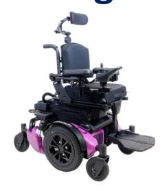
**Description**: Alltrack P3 MWD power wheelchair. Base width: 535mm. Base length: 890mm. Seat to floor height: 445mm. Turning radius: 510mm. Speed: 10km/h. Battery capacity: 50amps. Selections of: Power Tilt 50°, Tilt and Seat elevate 11in, Tilt and recline with mechanical shear reduction seating functions.
