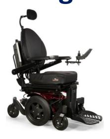
**Description**: Q500 Mini MWD Powerchair. 13in Drive Wheels. 7in Castors. 50 Ah Batteries. 10km Speed. 30km Range. Selections of: 50 Degree Posterior Tilt. 30cm Seat Elevate. 130 Degree Recline. Power Centre-mount (PCM) Elevating & Articulating Leg rests with Dual Flip Up Footplates or Removable Manual/ Power Swing Away (PSA) Elevating Leg rests with Angle Adjustable Footplates, swings In/Out. Calf Pads Included.
