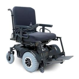
**Description**: A bariatric powered mobility solution with the necessary options and sizing to accommodate heavy duty requirements. 14in Drive Wheels. 9in Solid Castor Wheels. Min Seat to Floor Height 16.5in. Maximum Rate Slope 6°. Max Speed 7km/h. Front-Wheel Drive. Q-Logic 3 Expandable Electronics. Swing Arm Suspension. High Efficiency And Mileage. 4 Pole Motors. Heavy Duty Capabilities. Selections of: Power tilt. Tilt and Recline.
