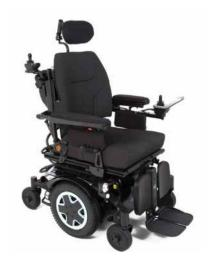
**Description**: TDXSP2 Heavy Duty Wide Mid wheel drive (MWD) base. Selections of: Tilt, Tilt and elevate, Tilt and recline seating functions. Non-expandable joystick. Optional Centre-mount or 70 Degree Swing away leg rests.
