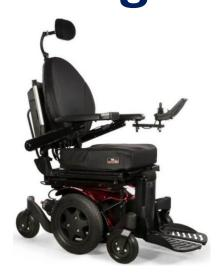
**Description**: Q500 Mini MWD Powerchair. 13in Drive Wheels. 7in Castors. 50 Ah Batteries. 10km Speed. 30km Range. Selections of: 50 Degree Posterior Tilt. Tilt and 30cm Seat Elevate. Tilt and 130 Degree Recline. Single Flip Up Centre-mount (CM) Footrests or Manual Swing Away (SA) Footrests with Angle Adjustable Footplates.
