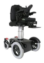
**Description**: TA iQ Junior Front Wheel Drive (FWD) power wheelchair. Base width: 600mm. Base length (without footplates): 820mm. Seat to floor height: 380mm. Turning radius: 450mm. Speed: 12.5km/h. Battery capacity: 80amps. Selections of: Tilt 45°, Tilt and elevate 11.8in, Tilt and recline with mechanical shear reduction.
