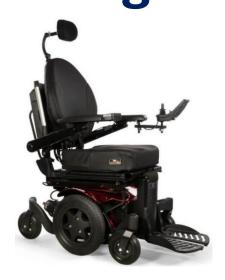
**Description**: Q500 Mini MWD Powerchair. 13in Drive Wheels. 7in Castors. 50 Ah Batteries. 10km Speed. 30km Range. Selections of: 50 Degree Posterior Tilt. 30cm Seat Elevate. 130 Degree Recline. Power Centre-mount (PCM) Elevating & Articulating Leg rests with Dual Flip Up Footplates or Removable Manual/ Power Swing Away (PSA) Elevating Leg rests with Angle Adjustable Footplates, swings In/Out. Calf Pads Included.
