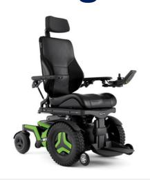
**Description**: Permobil F3 Mid-Wheel-Drive Power Wheelchair with selections of Power Tilt, Power Elevate, Power Recline and Power Centre-mount (PCM) Elevating Leg rest. Max Speed 10km/h, 14in Drive Wheel, Floor-to-Seat Height - 17.5-19.5in. Selections of: 50° Power Tilt, 12in Power Elevate, 180° Power Recline, 170° Power Elevating Leg rest.
