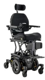
**Description**: The narrowest, most compact and manoeuvrable power base in the Quantum range. 14in Drive Wheels. 5in Solid Castor Wheels Front. 6in Solid Castor Wheels Rear. Min Seat to Floor Height 17.5in. Maximum Rate Slope 6°. Max Speed 10km/h. Mid-Wheel Drive (MWD). Q-Logic 3 Expandable Electronics. SRS Suspension. High Efficiency And Mileage. 2 Pole Motor. Fender lights. Selections of: Power tilt, recline, elevate (TRE), power elevating centre mount (PCM) leg rest.
