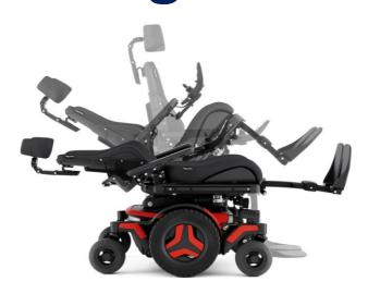
**Description**: Permobil M3 Mid-Wheel-Drive Power Wheelchair with selections of Power Tilt, Power Elevate, Power Recline and Power Centre-mount (PCM) Elevating Leg rest. Max Speed 10km/h, 14in Drive Wheel, Floor-to-Seat Height - 17.5-19.5in. Selections of: 50° Power Tilt, 12in Power Elevate, 180° Power Recline, 170° Power Elevating Leg rest.
