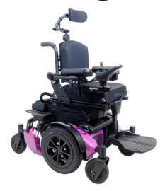
**Description**: Alltrack P3 Mid Wheel Drive (MWD) power wheelchair. Base width: 535mm. Base length: 890mm. Seat to floor height: 445mm. Turning radius: 510mm. Speed: 10km/h. Battery capacity: 50amps. Selections of: Power Tilt 50°, Power elevate 11in, Power recline with mechanical shear reduction seating functions, and Powered centre mount (PCM) elevating and articulating leg rest with flip-up, angle adjustable footplates.
