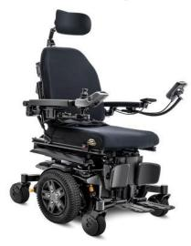
**Description**: A Mid Wheel Drive (MWD) powerchair, easy to customise the mechanical and electronic set up. Ideal for home and in the community. 14in Drive Wheels. 6in Solid Castor Wheels Front. 6in Solid Castor Wheels Rear. Min Seat to Floor Height 16.5in. Maximum Rate Slope 7.5°. Max Speed 10km/h. Selections of: Power tilt. Power tilt and elevate. Power Tilt and Recline.
