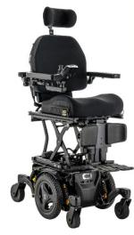
**Description**: The narrowest, most compact and manoeuvrable power base in the Quantum range. 14in Drive Wheels. 5in Solid Castor Wheels Front. 6in Solid Castor Wheels Rear. Min Seat to Floor Height 17.5in. Maximum Rate Slope 6°. Max Speed 10km/h. Mid-Wheel Drive (MWD). Q-Logic 3 Expandable Electronics. SRS Suspension. High Efficiency And Mileage. 2 Pole Motor. Fender lights. Selections of: Power tilt. Power tilt and elevate. Power Tilt and Recline.
